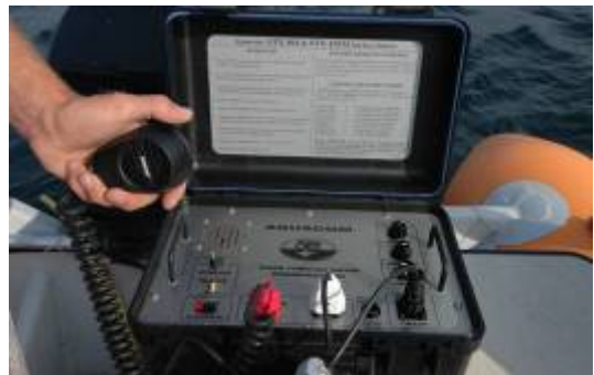
1 station surface munie d'un hydrophone
