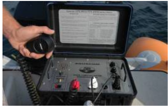
1 station surface munie d'un hydrophone
